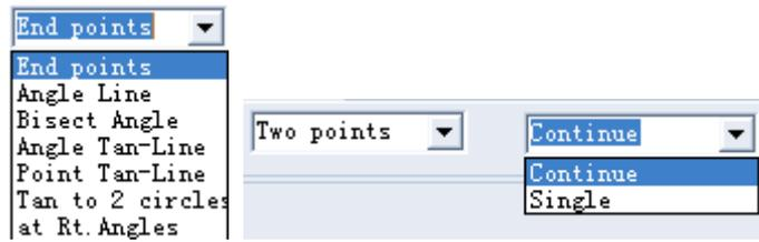
If the chosen operation needs interactive input of relevant parameters, please input related parameters in “parameter interactive sector” (numerical values such as length, angle and radius and so on) (as shown in the following figure).
